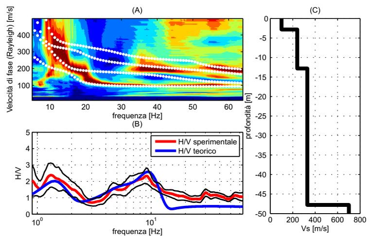
Figure 3. Joint fit of H/V and dispersion curve
