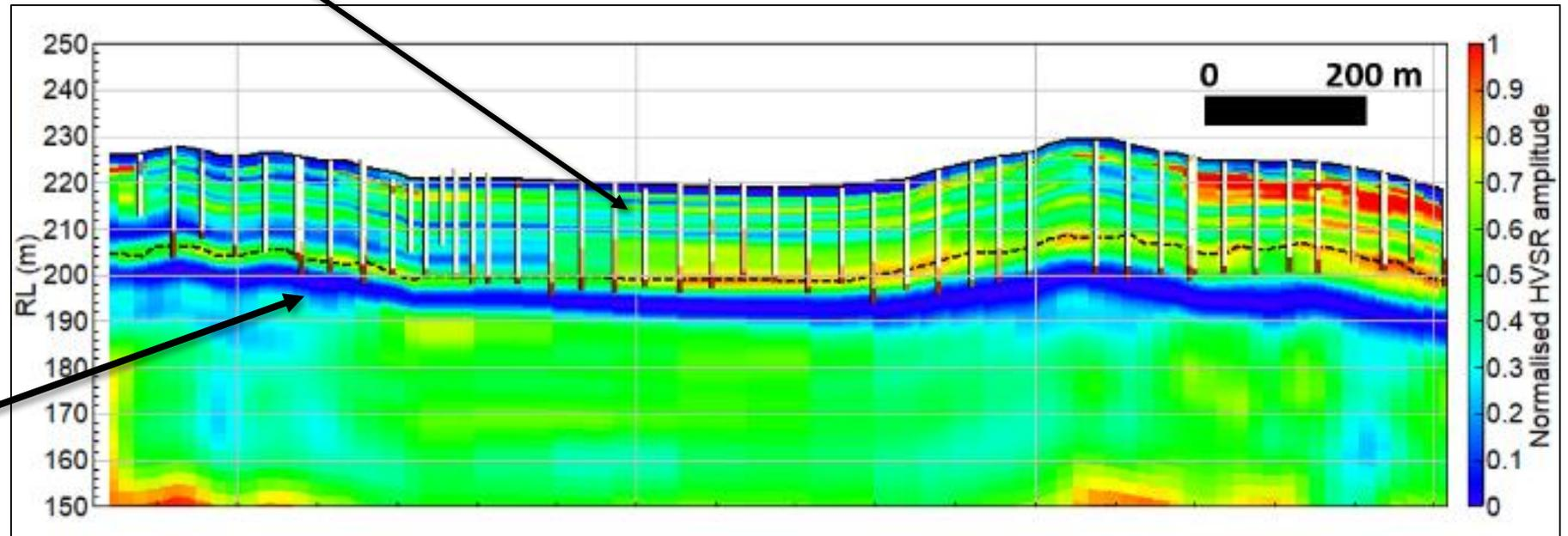
The Chegan clay unit intersected the near end of drillholes (brown) provides an anomalous HVSR low response – marker horizon. Velocity inversion from clay band could also be produced in a shallow coal basin to track coal seams.
