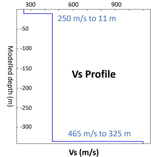
Using passive seismic data and drillhole data from nearby Snapper deposit
