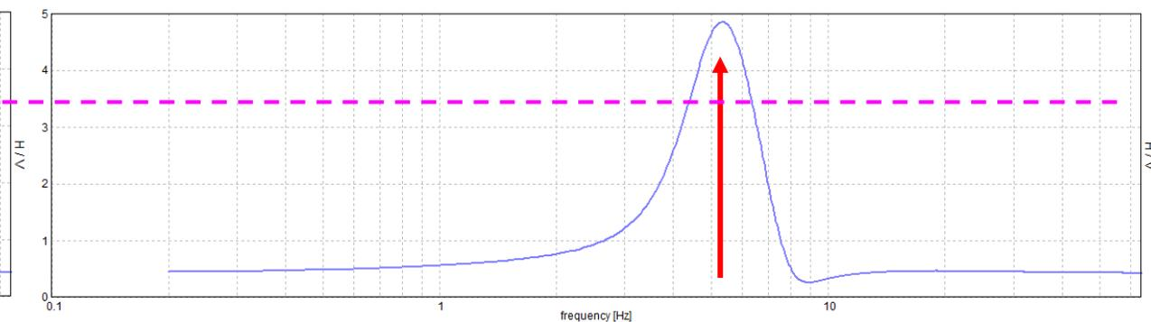
Increased HVSR peak frequency amplitude due to higher density of layer 2
