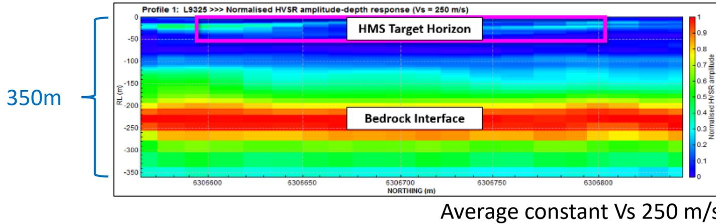
Basement interface depth is likely under-estimated when using a constant average  $V_s$  of 250m/s, because modelled velocity for 2<sup>nd</sup> layer is 465m/s
