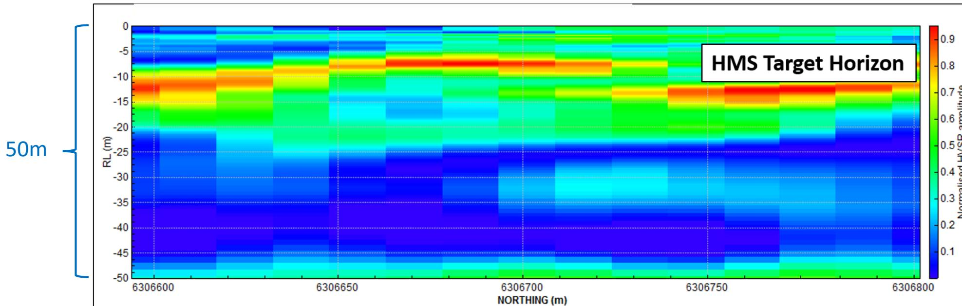
Multiple shallow dipping interfaces identified in the HMS deposit zone
