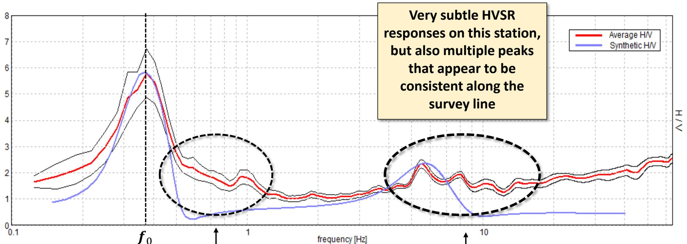
HVSR anomaly peaks sitting above  $f_0$  – gradational weathering into acoustic basement layer, limestone?
