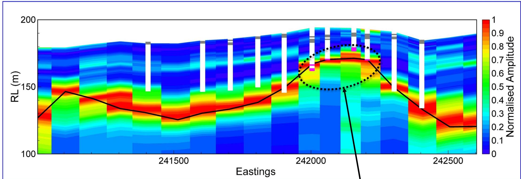
These drillholes intersected granite-gneiss bedrock towards the end of hole, whilst the other drillholes along this survey line did not intersect basement.
