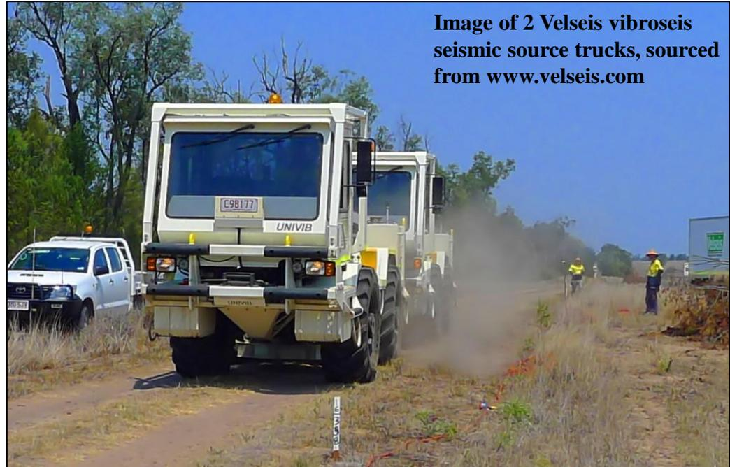
Image of 2 Velseis vibroseis seismic source trucks, sourced from [www.velseis.com](http://www.velseis.com)
