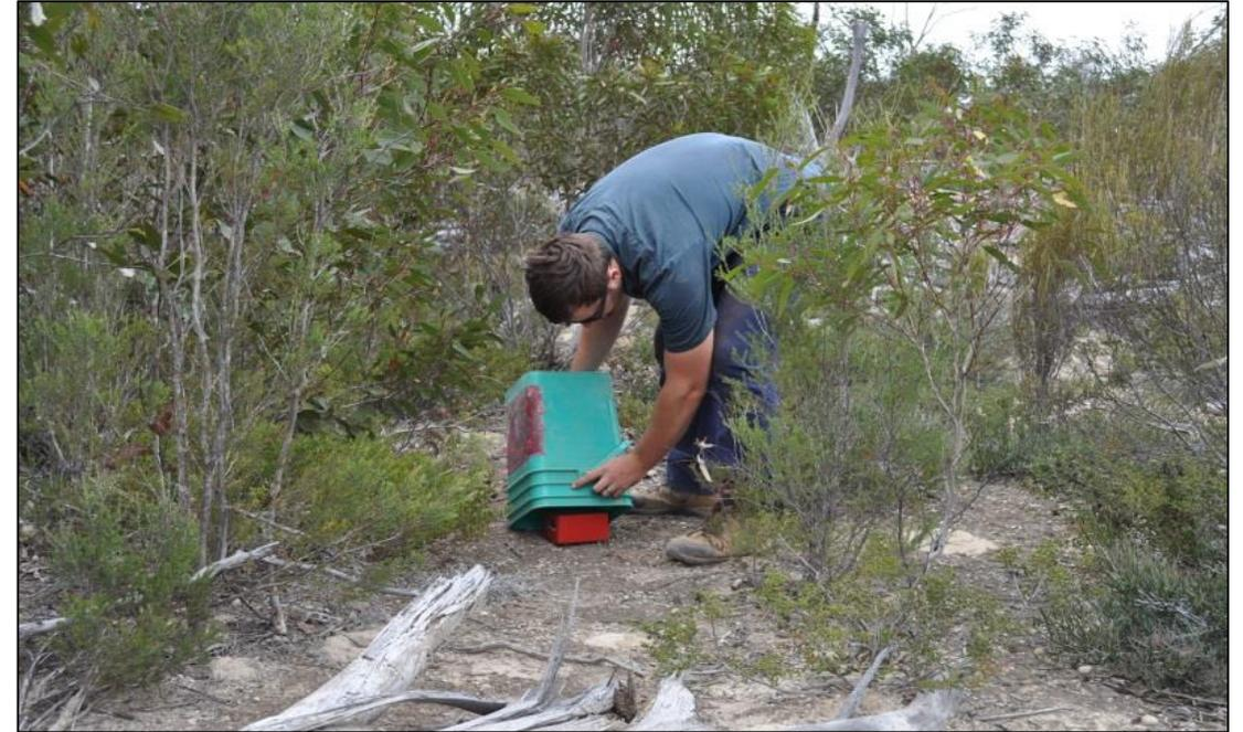
**HVSR passive seismic data acquisition using a Tromino<sup>®</sup> seismometer**
