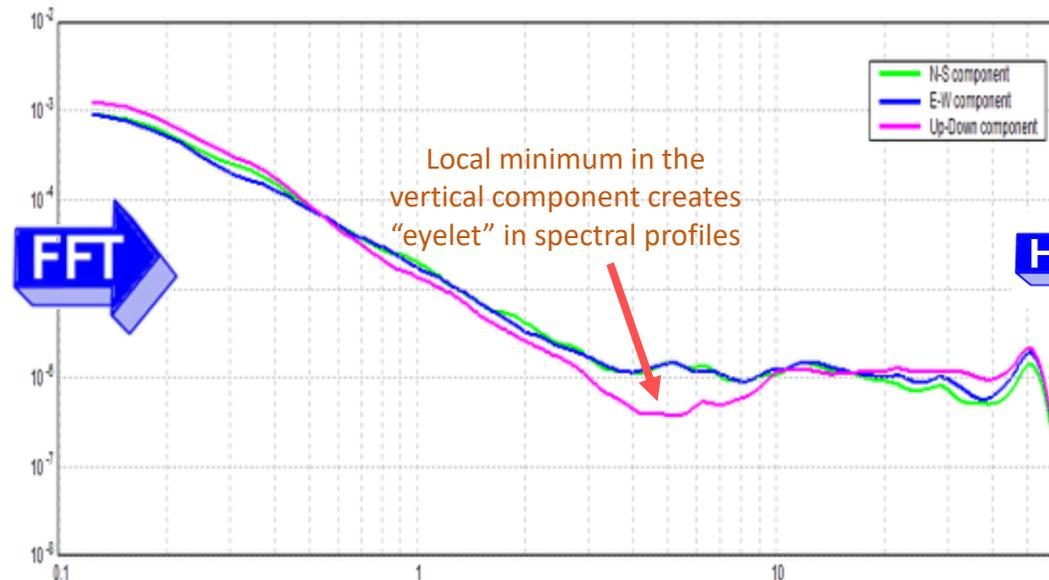
Frequency power spectrum of ambient vibrations
