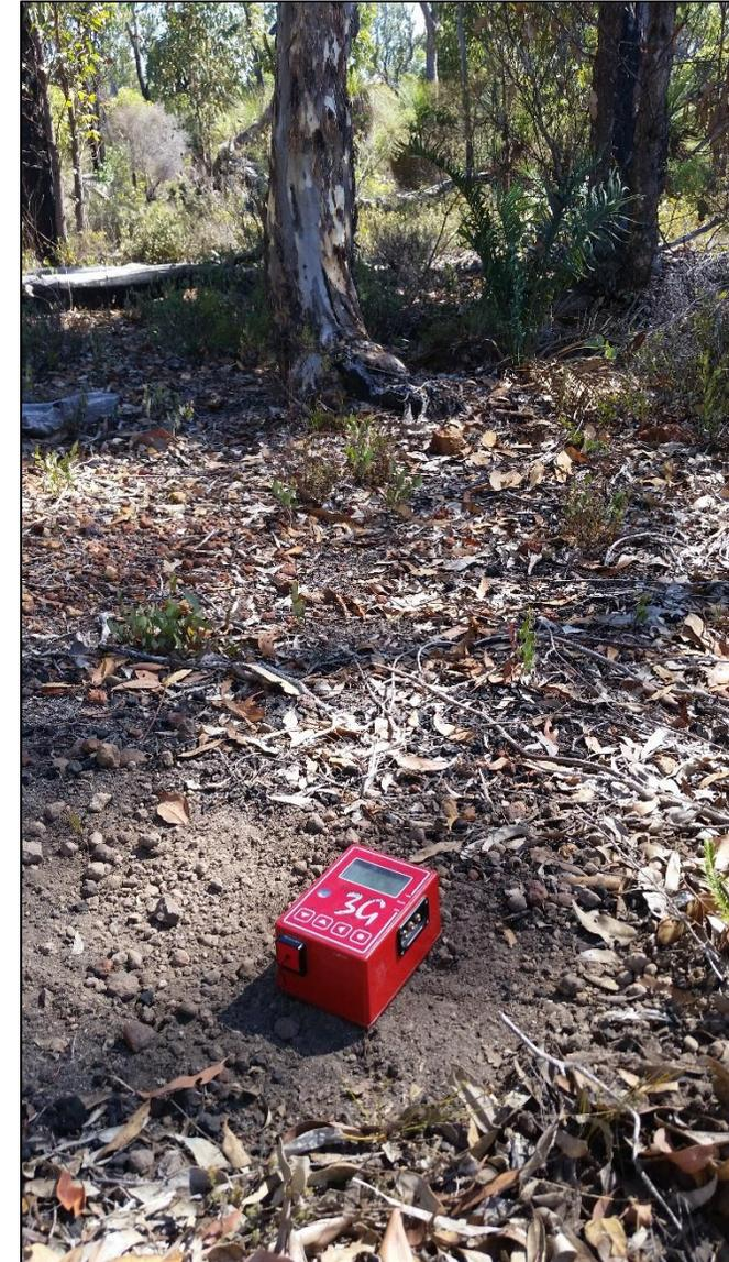
HVSR passive seismic surveying in the Wilga Basin
