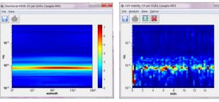
**VIBRATION ANALYSIS.** Sorting and spectral analysis of signal sections above thresholds, according to the European regulations on strong vibrations in structures. Automatic editable reports including tables and figures.
